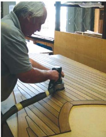
Construction of a Moody off-boat deck is a precision process, carried out by a mixture of the latest high-tech machinery and highly skilled craftsmen. For standard production boats, the teak strips are produced by CNC machine following design by
