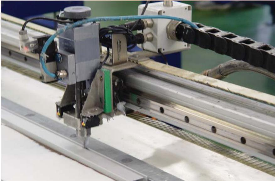
*Automatically applying the silicone*
