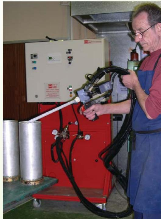
Dispensing the resin into moulds
