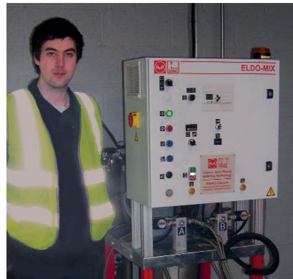
Sales Manager for Polyurethane Moulded Products, Mark McKeown with the DOPAG ELDO-MIX 101 used for producing a variety of integral skin mouldings
