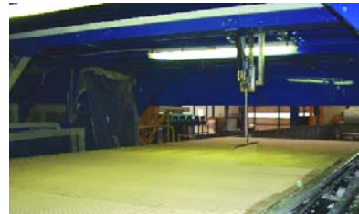
Dispensing polyurethane onto the panels with the multi-nozzle applicator
