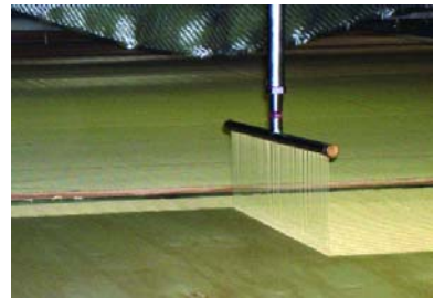
Dispensing polyurethane onto the panels with the multi-nozzle applicator
