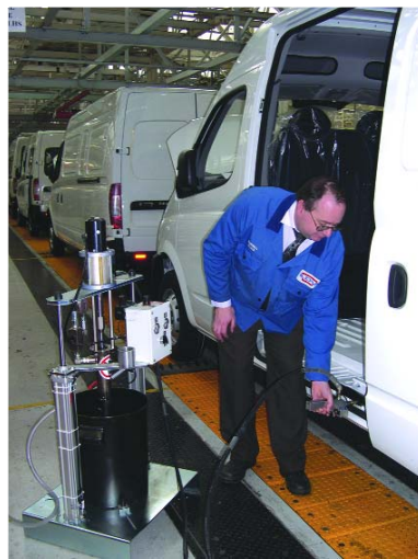
Applying the grease with the specially designed nozzle
