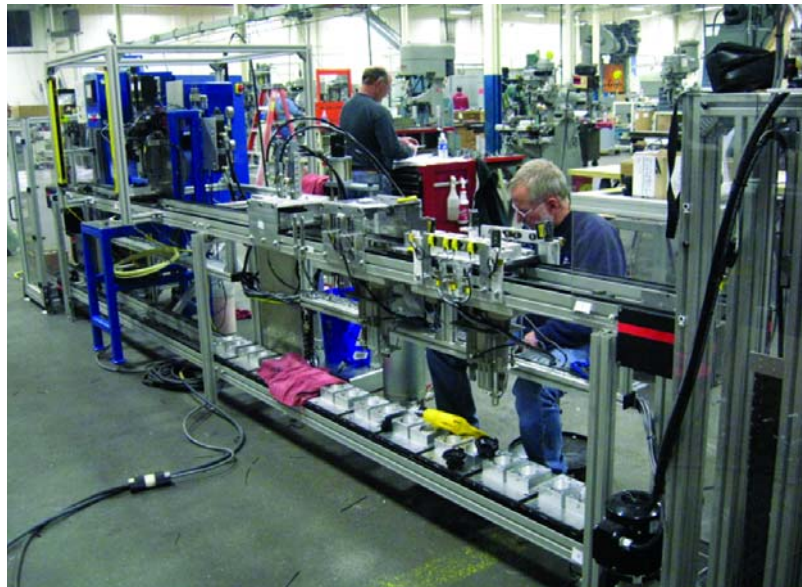
The grease dispensing section of the assembly line under construction
