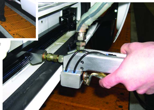
Applying the grease with the specially designed nozzle
