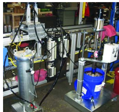
Oil feed and grease pumping systems
