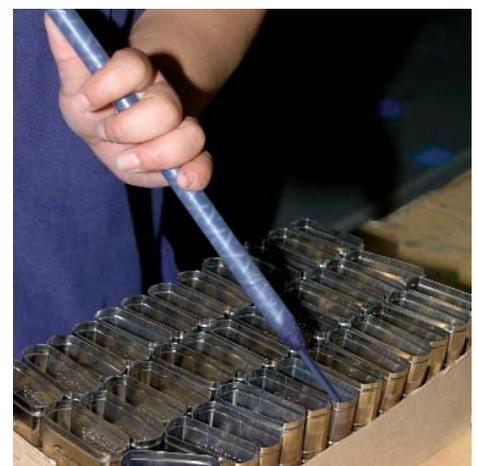
Dispensing the mixed epoxy resin into the paint brush ferrules via a disposable plastic static mixer
