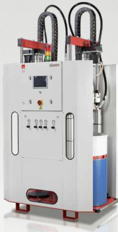
The silcomix is a compactly designed, electrically driven piston pump, metering and mixing system. It is used for continuously processing medium to high-viscosity, silicone-based media with a mixing ratio of 100:100.
