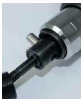
Quick change system for the mandrel.
