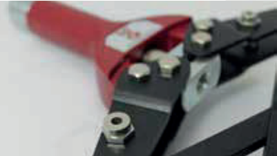
Replaceable nosepieces screwed into the tool.
