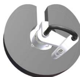
SCARA robots: kidney-shaped envelope with dead space
