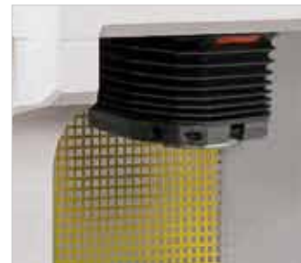
Round Ram locked against Rotation with TDC switch (74/76) or position measuring system (374/376) on the rotational guide rod.
