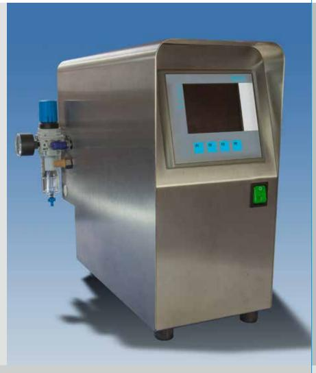
The control unit CU30 is a PLC for hand and stationary screwdriving systems - including our feeding systems. It allows our customers to scale the system within simple or complex assembly tasks. Due to the modular design a maximum flexibility for different requirements is available. Operation of the control unit happens via a convenient touch screen panel (optional outsourced version available).
