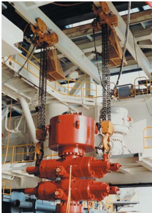
BHS100M (100-ton system) in the process of deploying Blowout Preventer stack
