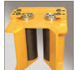
Pressure sensing guide rollers
