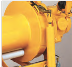
Automatic drum brake
