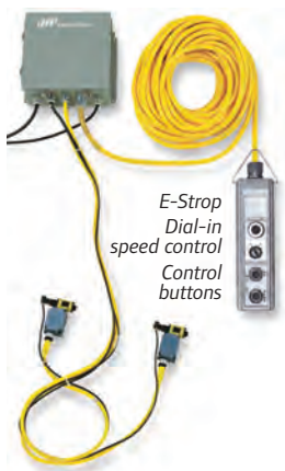
Optional pendent for secondary local control
