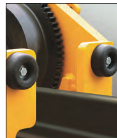
Trolley guide rollers, rubber bumpers & rail sweeps
