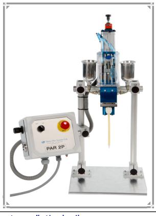
An extensive range of metering pump sizes and low volume disposable static mixing nozzles ensures that the PAR2-P can be tailored to suit most application requirements handling material mix ratios from 1:1 to 18:1.
