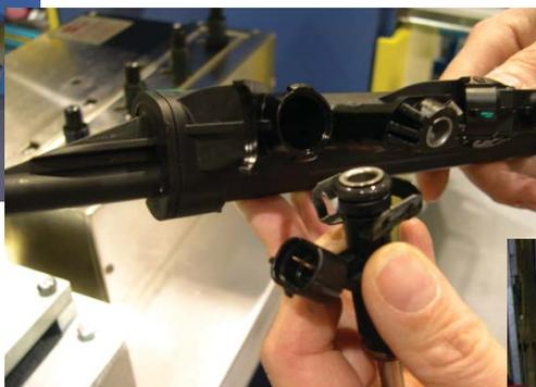
Assembling the injector into the fuel rail
