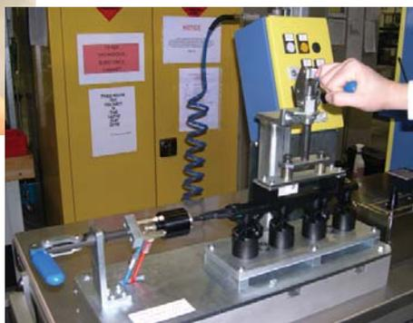
Testing the assembled fuel rail for leaks
