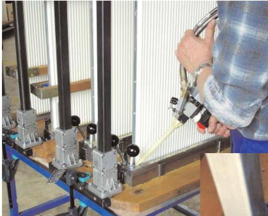
*Mixed resin being dispensed into the fixture*
