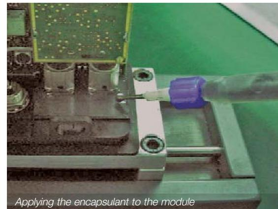
*Applying the encapsulant to the module*
