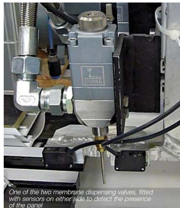
*One of the two membrane dispensing valves, fitted with sensors on either side to detect the presence of the panel*
