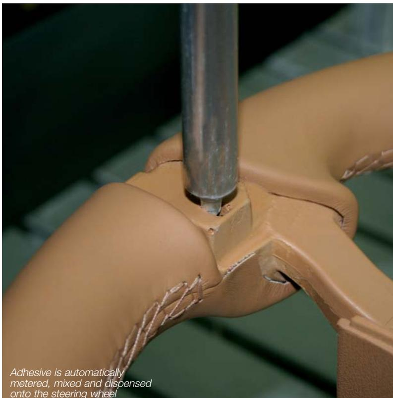
Adhesive is automatically metered, mixed and dispensed onto the steering wheel
