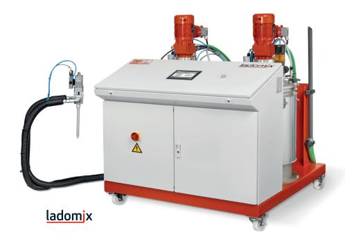
The ladomix G-SF is a compact mobile metering and mixing system with gear pumps pumps for laminating processses in the packaging industry. It can be used to dose and mix solvent-free, self-levelling two-component polyurethane laminating adhesives in a mixing ratio of 100:100 to 100:10. The material is then metered into the gap between the rollers of the laminating machine and applied to the outer film of the packaging. This is then bonded to the inner film.
