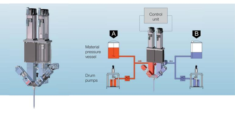
metamix is used to handle multi component materials. Due to its compatibility and modularity, two metadis single component piston metering systems, with different sizes if required, are used. They can be connected by simply using a mixing block onto the outlet of which a disposable plastic mixer is mounted.
