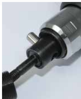
Quick change system for the mandrel.
