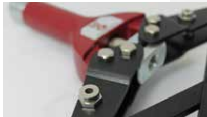
Replaceable nosepieces screwed into the tool.
