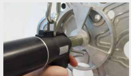
Special accessory angular adapter for keeping the needed rectangularity to the component.
