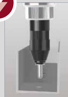
Retension nosepieces available as options ensure that the rivet cannot fall out of the tool even in vertical working position and that the mandrel is discharged after the setting process.
