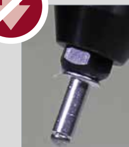
Retension nosepieces available as options ensure that the rivet cannot fall out of the tool even in vertical working position and that the mandrel is discharged after the setting process.
